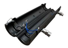
Aerial cable joint closure, also called self supporting aerial cable closure or aerial free breathing mechanical joint closure. It is free breathing and suitable for straight, butt, and branch splices of non-pressurized communication cables. The one piece construction permits complete splice access, without removal of the closure or bonding of the cables.
