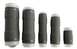
Cold Shrink Tubes are a series of open-ended, tubular rubber sleeves, which are factory expanded and assembled onto a removable core. They are supplied for field installation in this prestretched condition. The core is removed after the tube has been positioned for installation over an in-line connection, terminal lug, etc., allowing the tube to shrink and form a waterproof seal. The insulating tube is made of EPDM rubber, which contains no chlorides or Sulphur.
